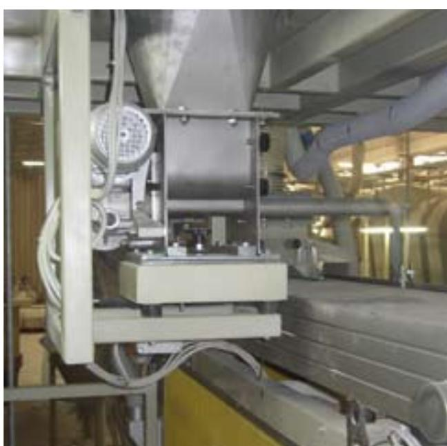
**MBF Micro-Batch Feeder for continuous volumetric feeding of powdery or granular materials** consist of a body entirely manufactured from stainless steel (optionally steel-reinforced SINT® engineering polymer), a horizontally mounted rotating agitator tool, a feeder screw beneath the agitator tool, a feeder pipe enclosing the protruding feeder screw, one drive unit each for agitator and feeder screw.
